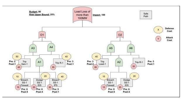
Here we see the attack/defense tree representation of the given power grid system. Each attack node is given a pre and post defense probability in addition to an attack and defense cost. The system is now given a budget and upper risk bound and an impact value to the system if compromised.
