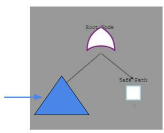
For the analysis algorithms to give correct output all diagrams must follow the format featured above. A tree's top level node, must be the Root Node component and it must have a Safe Path child node. The Safe Path node represents the likelihood that an attack doesn't occur or that the attacker fails on all attempts. You can begin constructing your system's tree at the same level as the Safe Path; your tree is represented by the blue triangle above.
